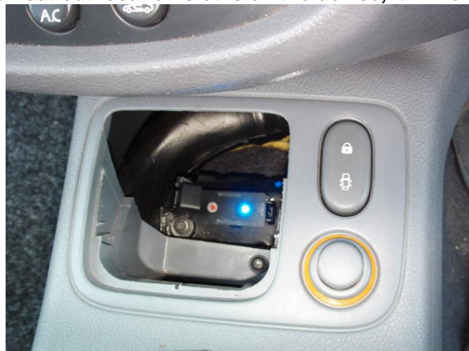
Plug bypass device into the socket
