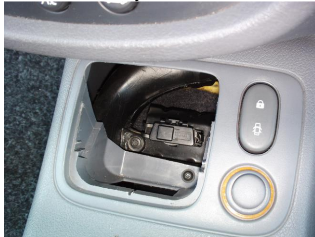
Remove the cover from the socket
