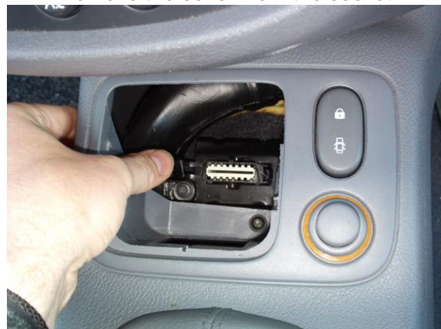
Plug bypass device into the socket
