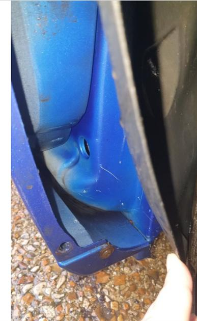
4, Slide foam insert back in – surprisingly easy. Push plastic liner back inside wing so that screw and clip holes align. Fit screw and do up tight. Ensure clip holes align, undo screw 2 turns, push clips in fully. Tighten screw fully and check clips are tight. All Done. Best done on a warm day when the plastic bends more easily.
