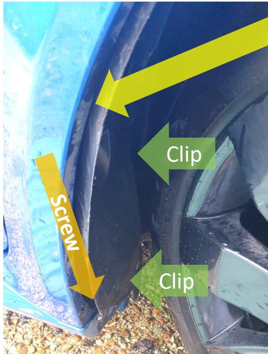
2, Pull the black plastic liner away from the wing until about level with top of wheel – no need to fully remove liner. Pull foam insert down and out.
