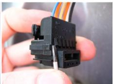
With the small plastic clip levered out slightly, you can now put the electrical screwdriver underneath the L shaped connector. Push the screwdriver in, and at the same time lever it upwards. The connector should simply click out of place and slide out the top of the connector block.
